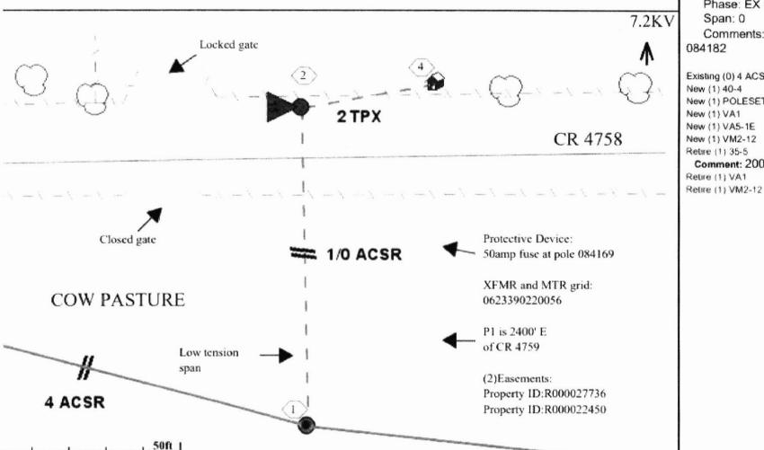
c. Remarks: Change out pole 084182 and build new overhead primary going N across CR 4758. Install (1) new primary pole, new 15kva r. and new overhead service to 200amp meterpole. Mbr will subfeed to future house. Meterpole ready. Requires (2)easements and Hopkins nty road crossing permit. XFMR and MTR grid: 0623390220056. Rate 1/ Rev 1. ATC due. CNR.
